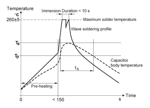
Ts: Capacitor body maximum temperature at wave soldering
