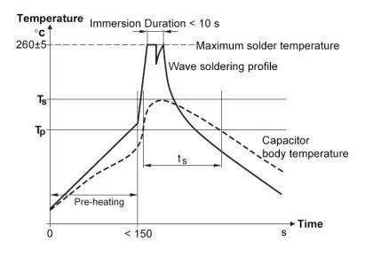
Ts: Capacitor body maximum temperature at wave soldering Tp: Capacitor body maximum temperature at pre-heating
